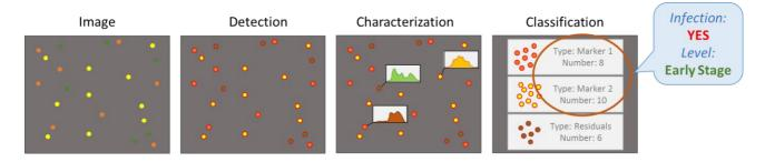
Since each plasmonic nanoparticle binds specifically to a biomarker of interest, it is possible to quantify the amount of each biomarker immobilized on the substrate by classifying and counting the different nanoparticles (Patent pending).
